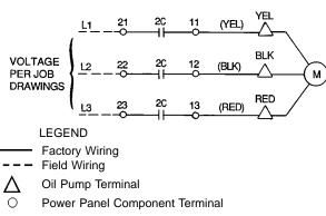
Fig. 30 — Oil Pump Wiring
